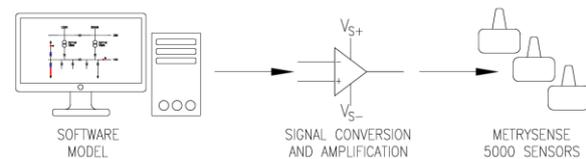
Fig. 11 HIL signal simulation for MetrySense type test at PNDC
