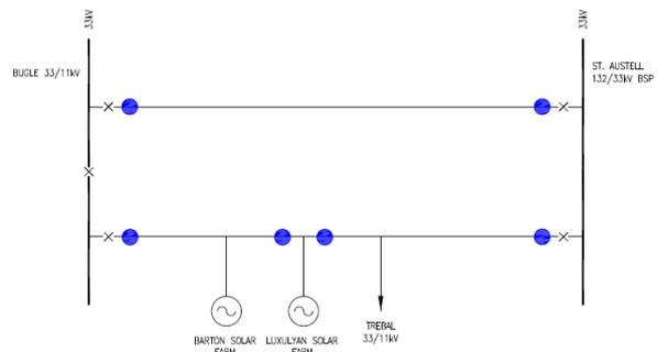
Fig. 4 Example of sensor location selection (blue circle) on 33kV network fed from St. Austell 132/33kV BSP
