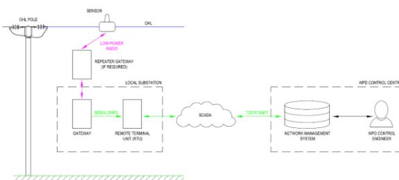
Fig. 3 Radio telecoms system architecture
