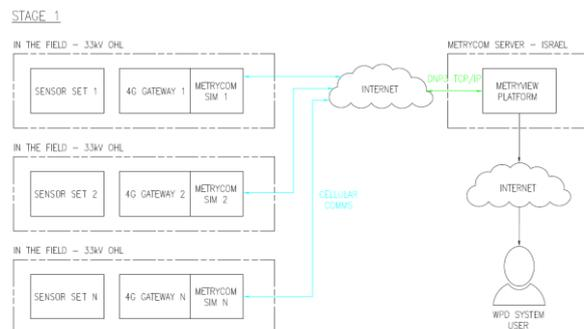
Fig. 8 Stage 1 works - cellular sensors relayed to Metrycom server in Israel while local server is built in UK
