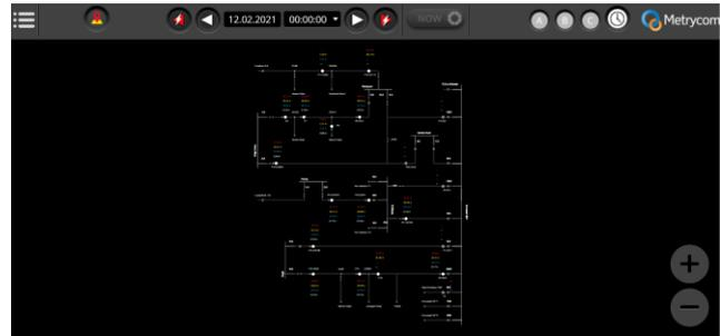
Fig. 7 Web-based MetryView GUI and SLD representation
