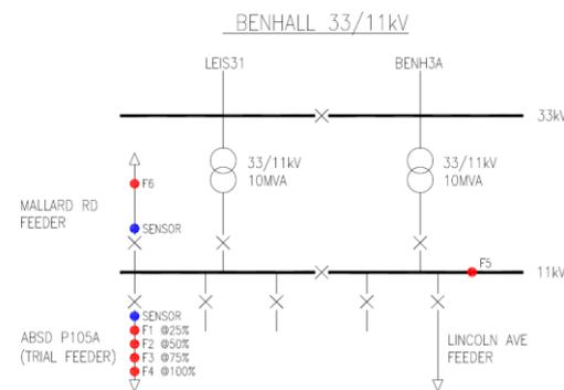
Fig. 12 Sensor and simulated fault locations at Benhall 33/11 kV substation for MetrySense type test at PNDC
