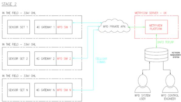
Fig. 9 Stage 2 works - cellular sensors migrated to Metrycom server in UK after completion of build
