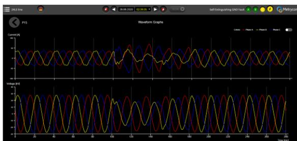
Fig. 10 Transient earth fault detected on St. Austell 33 kV network on 28 August 2020
