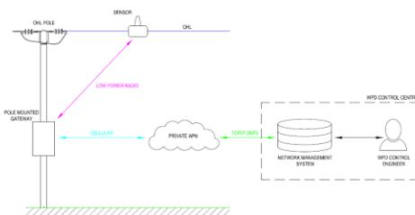
Fig. 2 Cellular telecoms system architecture
