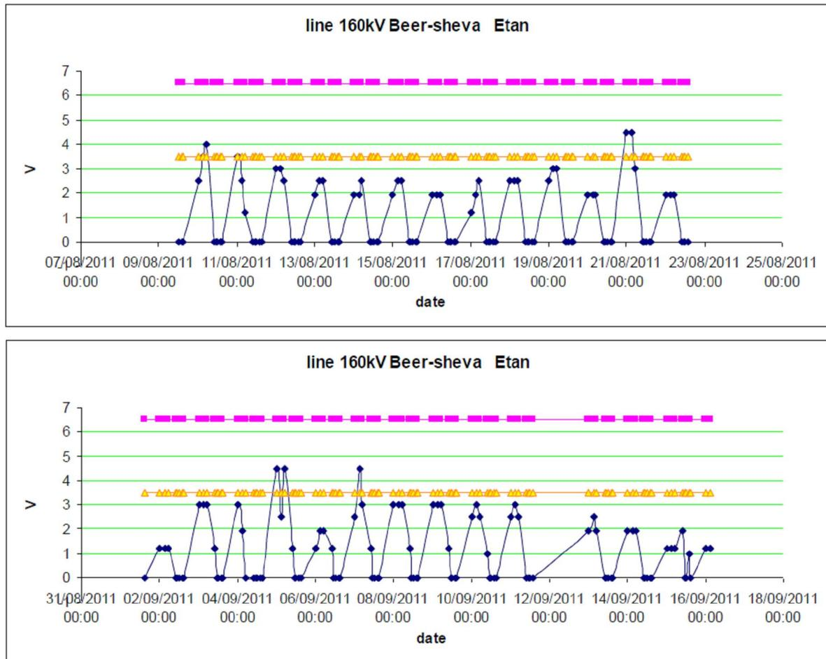
Fig. 10: Beer-Sheva Sensor results in August and September. The insulators were polluted, but the measurements were in the “Green” and “yellow” level, but did not cross the “red” level. Washing was therefore not required.
