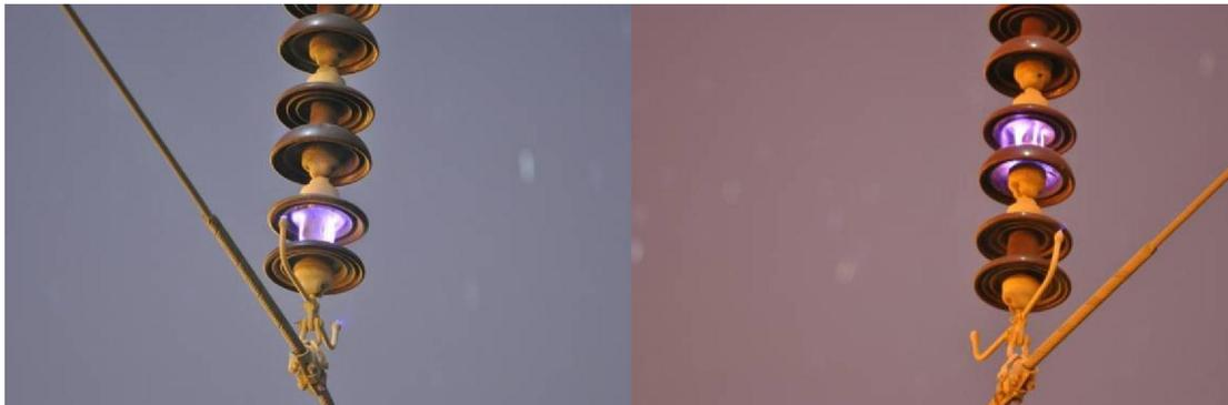
Fig. 2. Discharge on polluted insulators of a 160 kV line.
